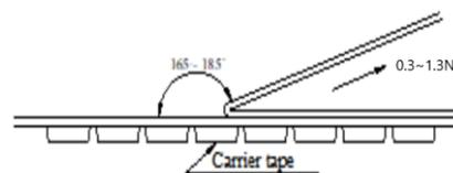
The peel speed shall be about 300 mm/minute
