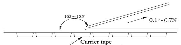
The peel speed shall be about 300 mm/minute
