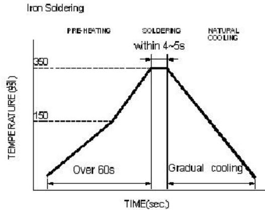
Iron Soldering times: 1 times max.
